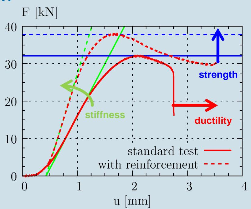
Load-displacement diagram for standard and reinforced specimens: typical changes in stiffness, strength, and ductility
