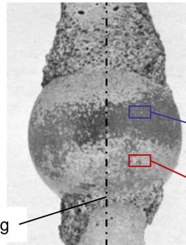
Inspection of post-failure fragments after failure under uniaxial compression of concrete [3] allows for a posteriori identification of two possible failure mechanisms for ITZ cracks:
