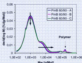
Figure 4: GPC results of bitumen.
