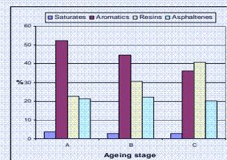
Figure 6: Generic fractions of bitumen.
