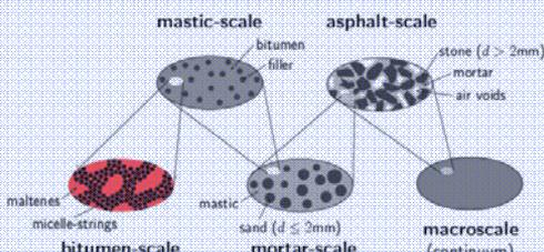
Figure 1: Observation scales introduced for multiscale modeling of asphalt.
