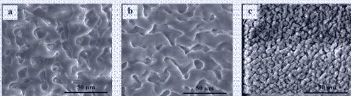
Figure 9: ESEM images of bitumen - original (a) and aged (b, c).
