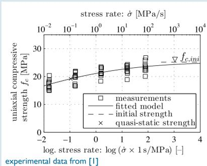
$f_{c,ini}$  ... initial strength of cement paste, prior to load-induced damage associated with creep deformation
